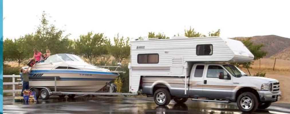
When towing behind a Lance camper, extending the hitch from the truck rearward to the camper bumper is necessary.
