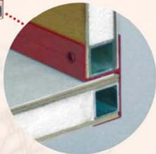
Our aluminum structural framing uses thicker, aircraft-grade .060-inch Alodine®-coated metal - welded within a precision jig system to ensure true-to-square, tight-tolerance assembly.
