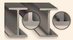
(Left) End view of Jayco's I-Class<sup>™</sup> structural steel chassis frame. (Right) End view of the welded I-beam frame used by many competitors that is subject to warping.
