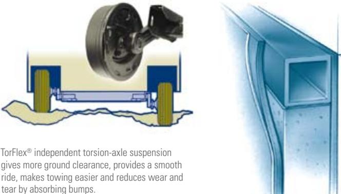
TorFlex® independent torsion-axle suspension gives more ground clearance, provides a smooth ride, makes towing easier and reduces wear and tear by absorbing bumps.
