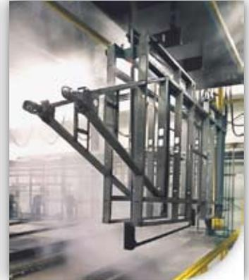
Corrosion-resistant frames are finished with a 12-stage E-Coat™ finishing system (select models).
