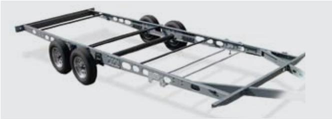
Jay Feather's ultra lite weight steel frame (EX-PORT and select EXP models) is 10-15% lighter and significantly more rigid than the frame of conventional travel trailers. Tapered rails place the strongest part of the frame over the axles. Instead of a welded frame, our modular frame design features "huck" bolt assembly and interlocking dimples.
