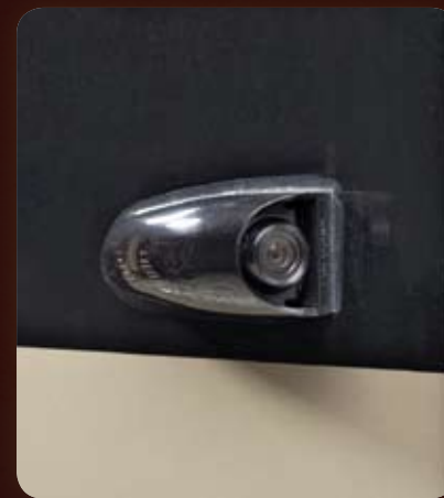
Side-View Cameras Available cameras are activated by the turn signals and viewed on the rearview monitor.
