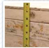
7" HEADER BEAM VS. 2" X 6" LUMBER
