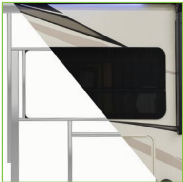
Aluminum Framing Around Windows in Sidewall
