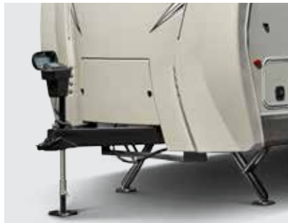
TRAVEL TRAILER ELECTRIC AUTO-LEVELING SYSTEM (BAL 5.3)
