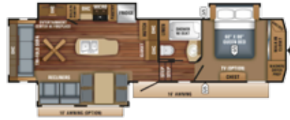
EAGLE FIFTH WHEEL | 321RSTS OPTIONS: A, E, F, G Ext. Lgth: 36' 11" Ext. Ht: 155" Unloaded Wt. (lbs): 10,300 Sleeps: 4-6
