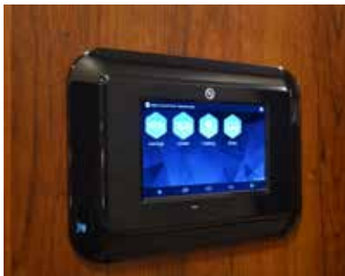
OPTIONAL WI-FI REMOTE CONTROL SYSTEM FOR SLIDE ROOMS, AWNING AND LIGHTING
