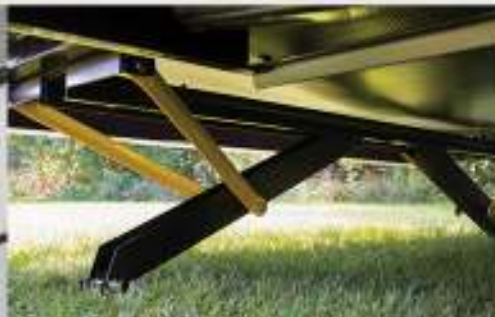
Electric Stabilizer Jacks All units now standard with electric stabilizers.
