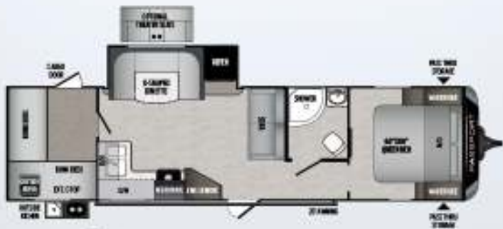
BEST IN CLASS 3100QB | Quad bunk w/ outside kitchen Weight: 6405 lbs | Length: 35' 11"
