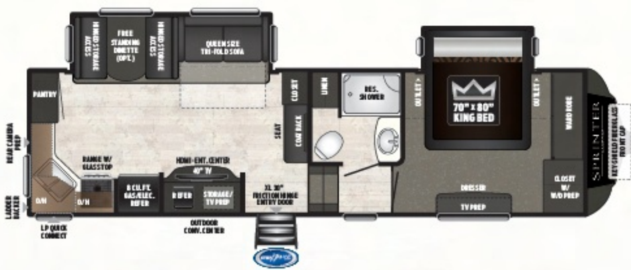
27FWML | Mid-living w/ king bed slide, w/d prep, floor-to-ceiling pantry, and o/s conv. center Weight: 8820 LBS. | Length: 31'10"
